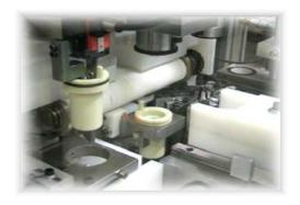
Fully automatic o-ring assembly machines available with automatic parts feeders, component positioning, o-ring insertion, o-ring assembly inspection, good / reject part gating, completed part counting, and more.
